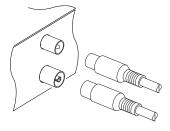
In this case, you will need to connect a cable from the RF OUT socket to the antenna connector on your television. To ensure your television can also pick up existing analogue channels as well, you will need to connect a cable from your television antenna or from the RF LOOP 2 OUT connector on the back of the digital receiver to RF IN connector.
